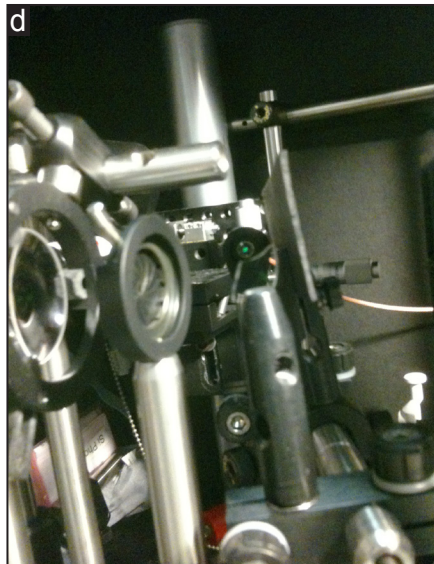
Illumination alignment: centering the reference beam on the reference photodiode
