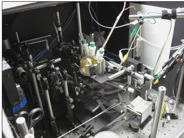
Figure D.12. Photoelectrochemical cell configuration , set up by Elizabeth Santori for characterizing n-type Si wire-array electrodes.
